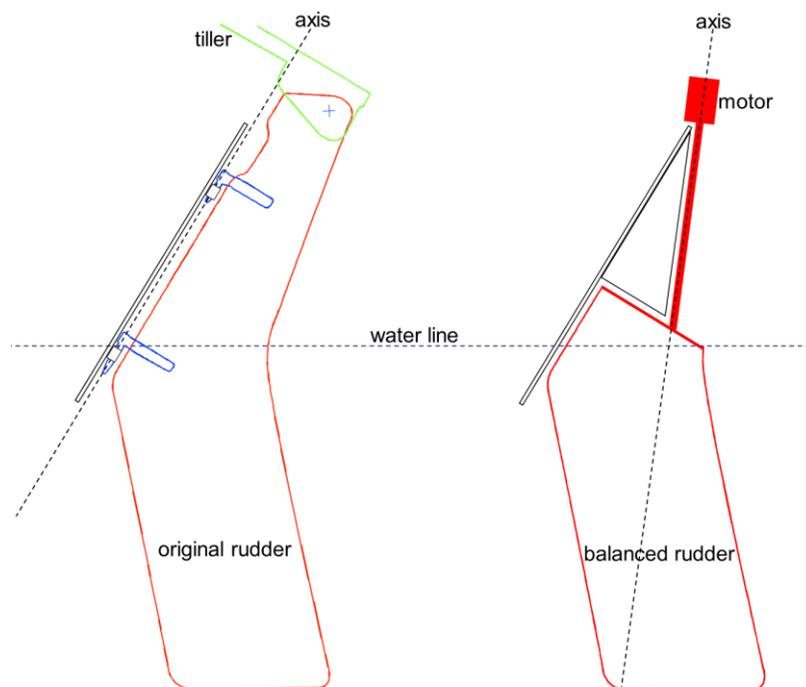
Figure 8 *Illustration of concept of balanced rudder*
