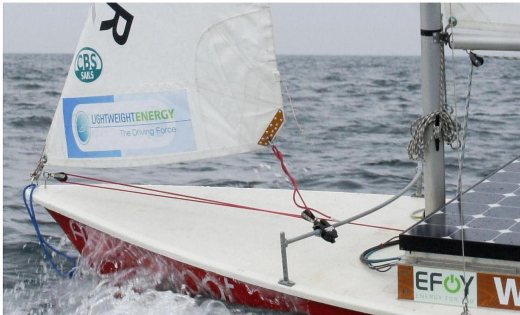
Figure 10 Self-tacking jib on ASV Roboat
