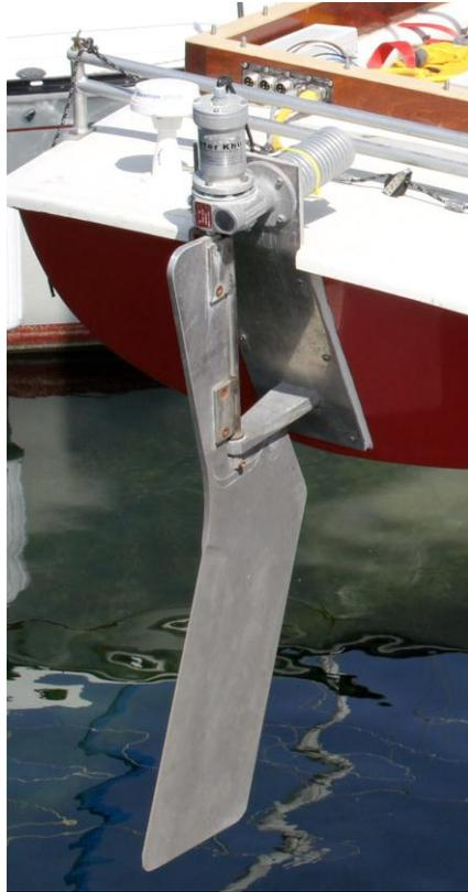
Figure 7 *Self-constructed rudder gear with balanced rudder (since 2008)*
