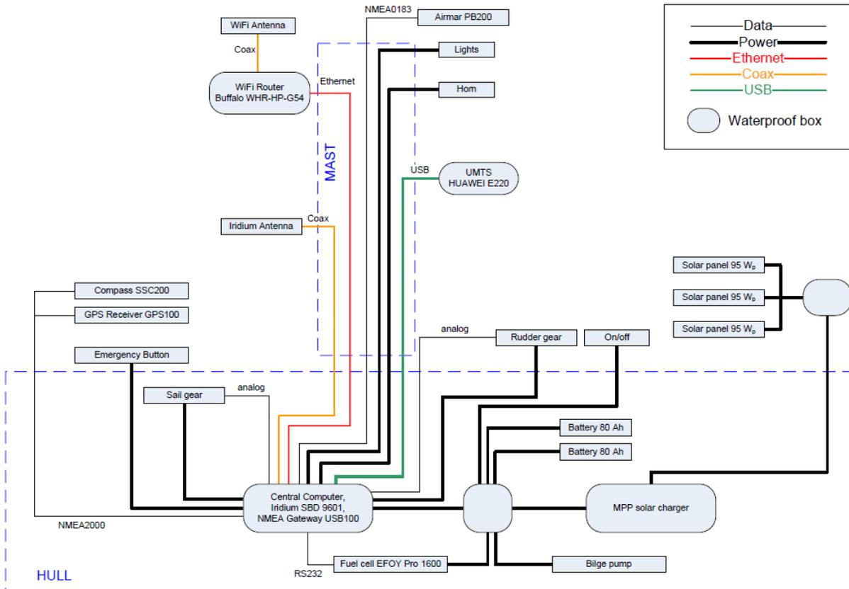
Figure 3 Technical infrastructure on ASV Roboat
