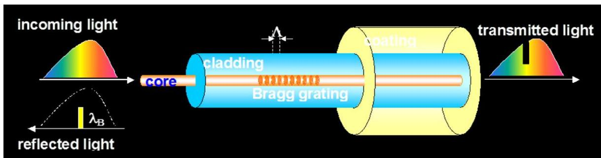
Fig 12: Schematic principle of optical fibre bragg grating strain sensors.
