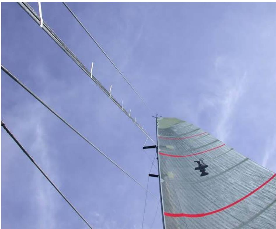
Fig 8: Twin, shaped carbon fibre runner cable on a V5 AC rig
