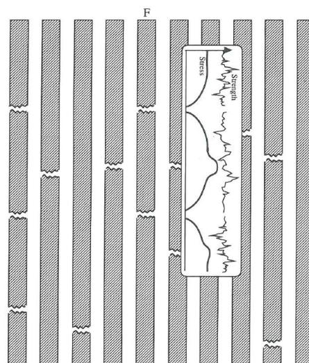
Fig 2: Schematic depiction of fractured fibres in a composite material. (Source: *An Introduction to Composite Materials*, D. Hull, T. W. Clyne)
