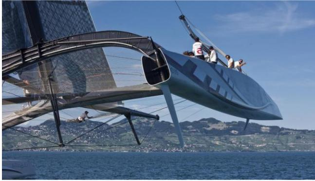
Fig 9: Alinghi V with high modulus carbon fibre spine rigging.
