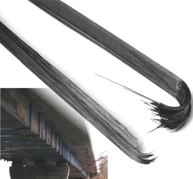
Fig 6: Consolidated composite tendon for shear strengthening purposes of concrete.
