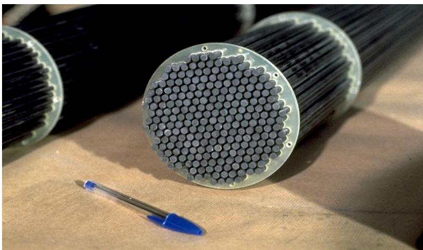
Fig 4: cross sectional view of a large bundled carbon fibre bridge cable.
