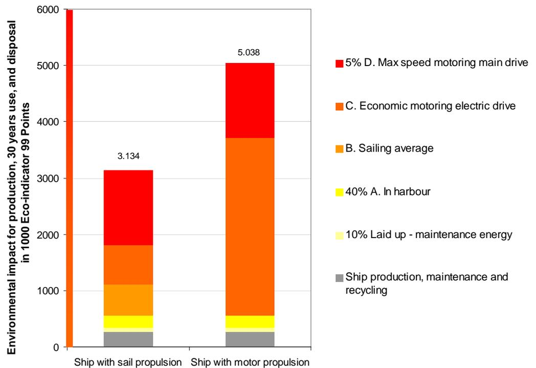
Figure 3 Environmental impact of the production, 30 years use and disposal expressed in Eco-indicator 99 points of a ship with sail propulsion, and a ship with motor propulsion
