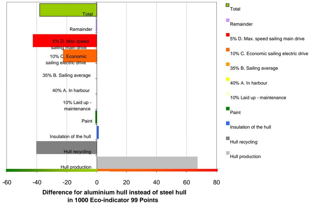
Figure 2 Difference in environmental impact as a result of choosing an aluminium hull instead of a steel hull, expressed in Eco-indicator points
