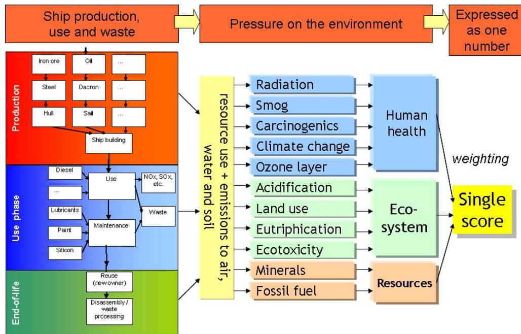
Figure 4 Schematic overview of calculation of Eco-indicator points
