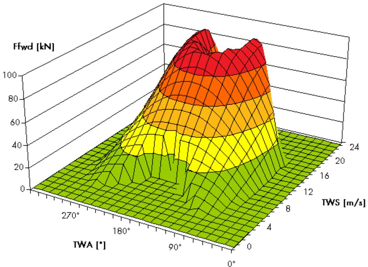
Above: Force mapping of SkySails propulsion for the SK160 kite system
