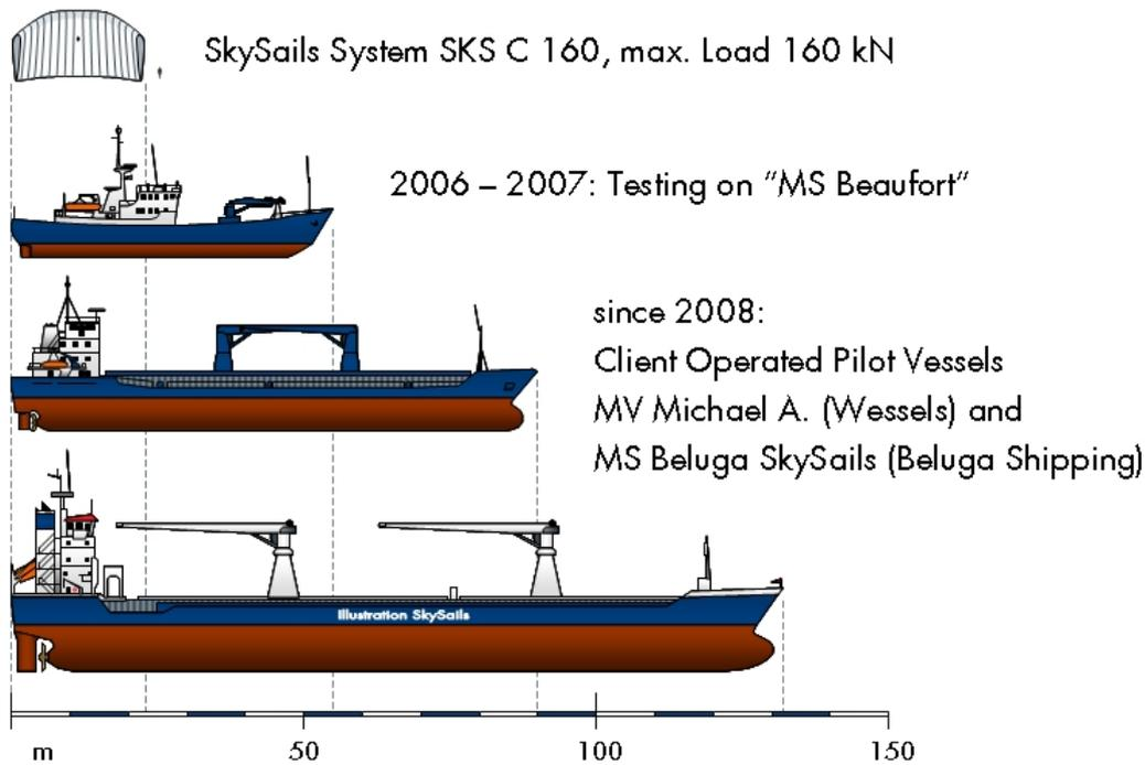
Above: Comparison of SkySails kite and vessel sizes
