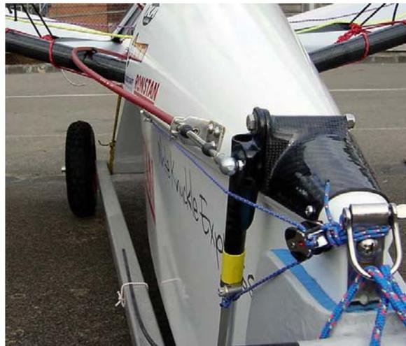
(a) Bow mounted wand sensor that tracks water surface and controls flap angle on forward hydrofoil. Photo by Hannah Kemlo.
