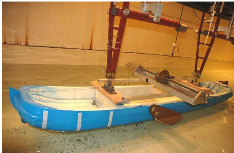
**Figure 2 Test setup, three single width carborundum strips are visible near the bow**
